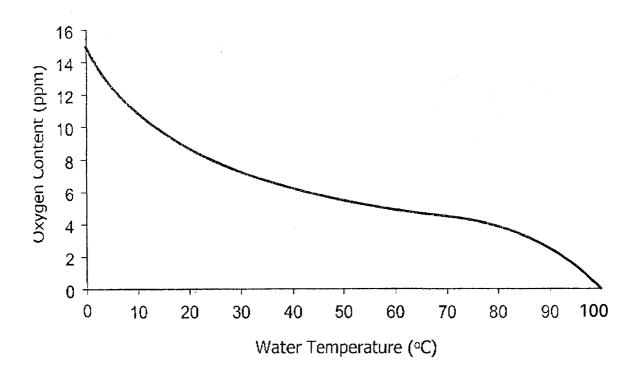
Feed water temperature in the mixing tank should be 80  $^\circ c$  to reduce oxygen to the boiler
